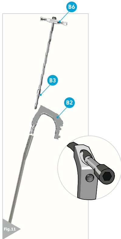
Combine (B2 Handle) with (ZFN) Use (B6 T Screwdriver) with (B3 Bar Aiming Holder Screw) and pass from (B2 Handle) screw hole and complete fixing with Nail (Fig. 11. )
